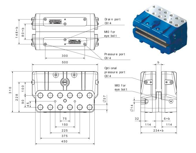
Stopping and/or holding brake for wind turbines
