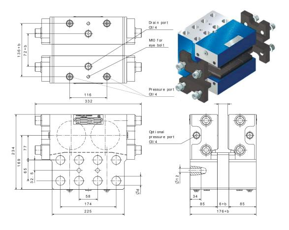
Stopping and/or holding brake for wind turbines
