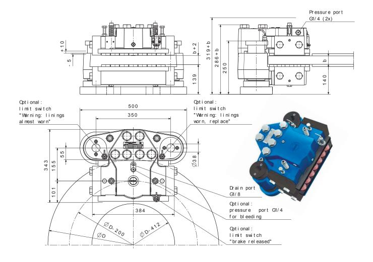
Stopping and/or holding brake for rotor of wind turbines
