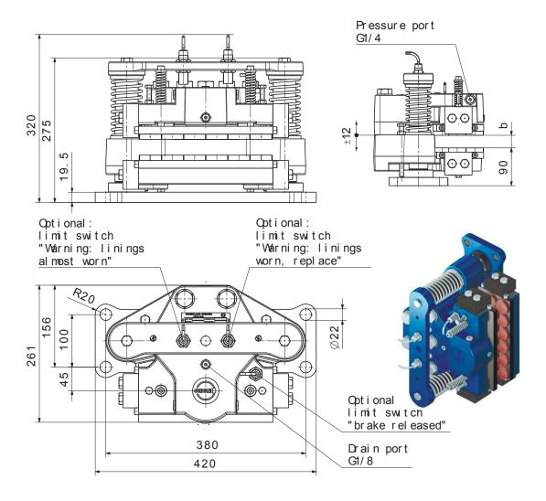
Stopping and/or holding brake for rotor of wind turbines
