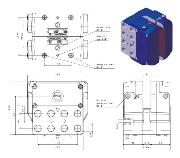
Stopping and/or holding brake for rotors of wind turbines
