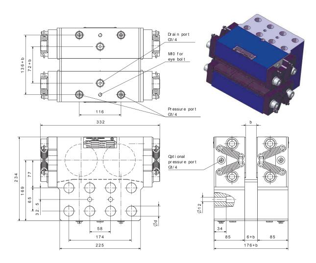
Stopping and/or holding brake for rotors of wind turbines
