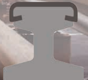
6000 Amp Welded Cap
