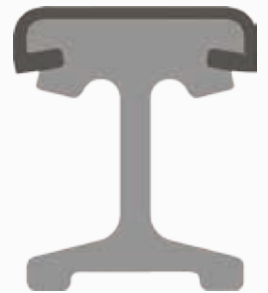
3800 Amp Welded Cap
