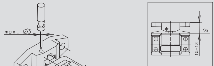
50 mm to direction of adjustment Actuator: metal
